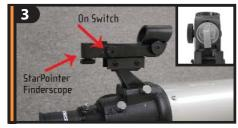
Now you will need to align the finderscope. Turn on the red LED light by turning the knob shown above. When used for the first time, remove the clear plastic disk that is located between the battery clip and the battery. See inset.
